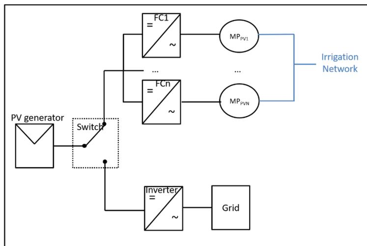
**Figure 5 - Mixed systems: the system is a PV irrigation system during the irrigation period, and a grid-connected system outside the irrigation period. The switch allows the change between the two operating modes and, in the case of this figure, the switch is in the PVIS position.**
