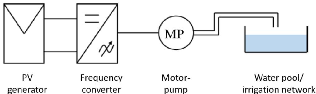
Figure 1 – Components of a PV irrigation system: PV generator, frequency converter, motor-pump and water pool.
