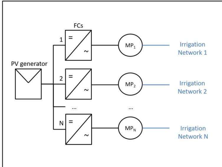
Figure 2 - Stand-alone PV irrigation systems: the irrigation system is fed by energy produced by PV generators. Figures depicted in black represent the electrical part, in blue the hydraulic part. FCs stands for frequency converters, while MP is for motor-pump.
