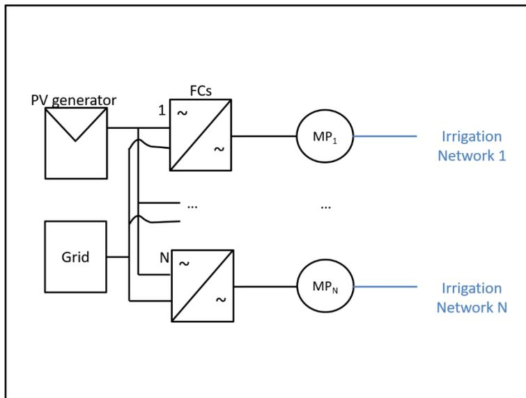
Figure 4 - Electric hybrid systems: hybridization among PV generators and the other sources is carried out in the electric part of the system.
