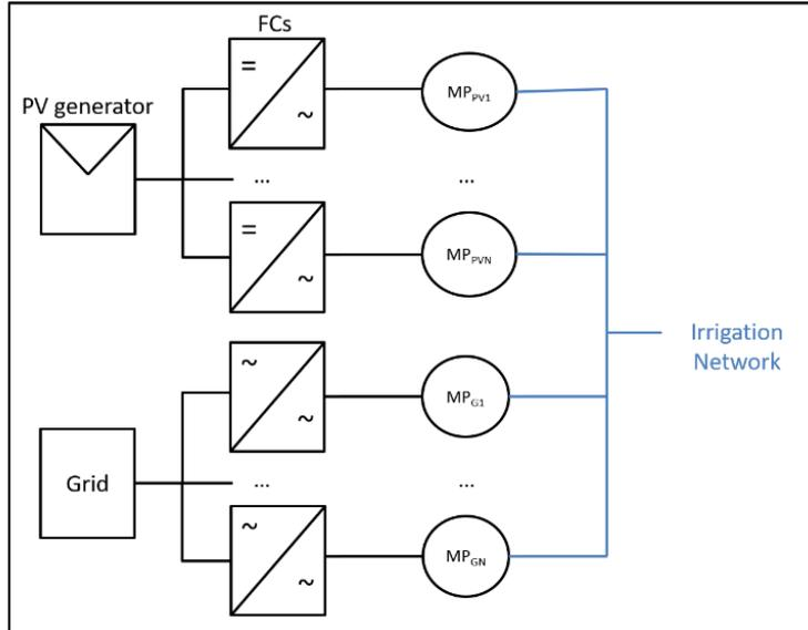
Figure 3 - Hydraulic hybrid systems: the irrigation system is fed by energy produced by PV generators but also from other sources (diesel or gas generator sets and conventional electricity grid), but hybridization is carried out into the hydraulic circuit.
